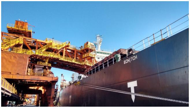
To prevent from walking under the shiploader boom and also jumping over tensioned lines at the main deck, a safe walkway connecting the superstructure to the upper accommodation ladder platform must be provided by The Master, by any available means such as painting, balustrades, hand railings and/or zebra tapes (black and yellow color), always through the main deck sea side in order to persuade and guide all persons to walk through a safer way;
